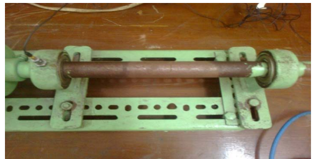
Fig. 3: Photograph of shaft installed with a piezoelectric sensor
